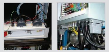
Field assembly time for devices and control cabinets is dramatically shortened using connectors instead of hard-wiring.
