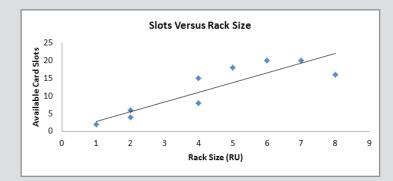
Trend between Number of Card Slots and Size of a Rack Mounted Chassis
