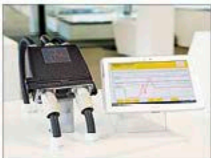
The data recorded and processed in the connector can be displayed both locally as well as made available to higher-order systems via the Cloud.
