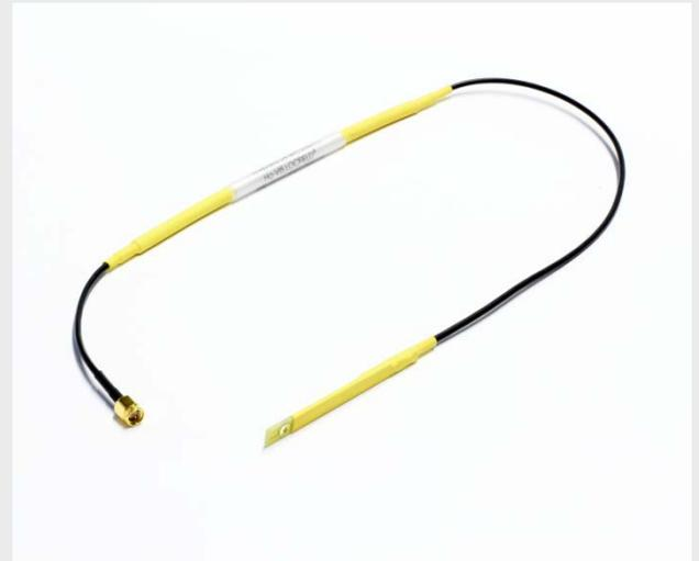
HARTING's Ha-VIS LocField traveling wave UHF antenna shows how new technology is expanding the reading zones and hence the flexibility of RFID in specific applications, like those involving doors and pass-through or small shelves.
