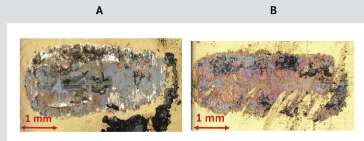
Figure 8: Hard gold flashed palladium-nickel (80/20) contact surface after 300,000 fretting cycles (A), hard gold contact surface after 900,000 fretting cycles (B) (performed at a digital microscope Keyence VHX 1000 D)
