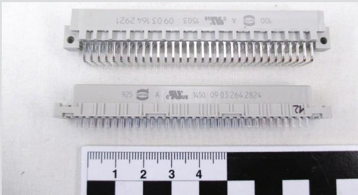
Figure 6: DIN-Signal type C male (top) and female (bottom)
