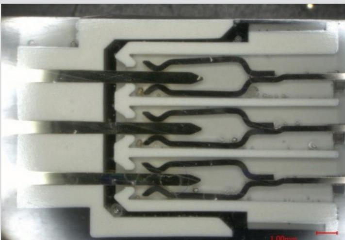
Figure 7: DIN-Signal type C female cross view
