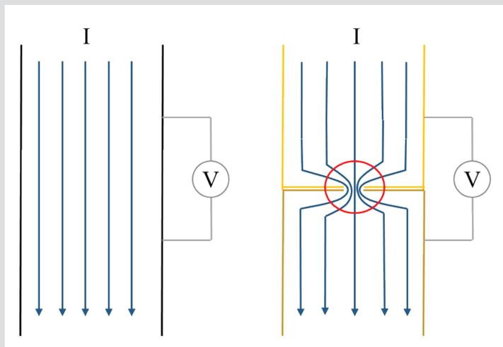
Figure 3: Schematic view of the current lines of a homogenous metallic conductor (left) and of a contact system with a circular effective contact area (right)
