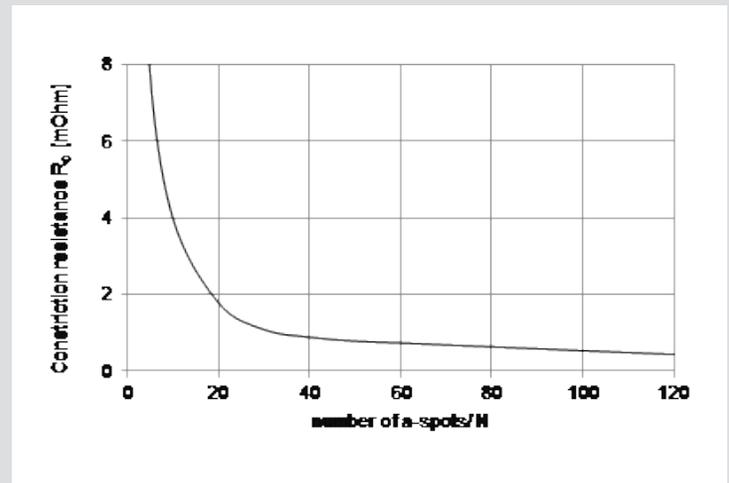
Figure 4: Constriction resistance in dependence of the number of a-spots
