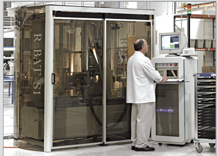
RoBAT tester performs AOI, continuity, and isolation testing
