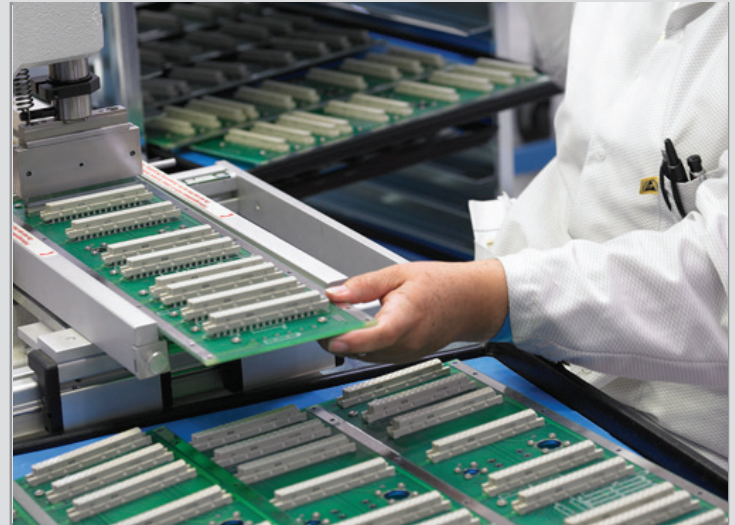
Backplane being assembled with a Press-fit machine
